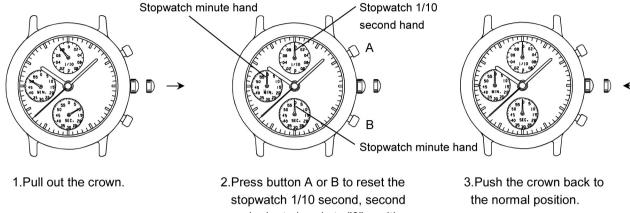
and minute hands to "0" position. \*By pressing button A set the stopwatch 1/10 second hand.
